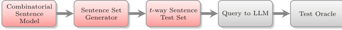
Fig. 2. An overview of the proposed testing approach. CT dependent steps are colored in red, LLM specific steps are colored in gray. (Color figure online)
