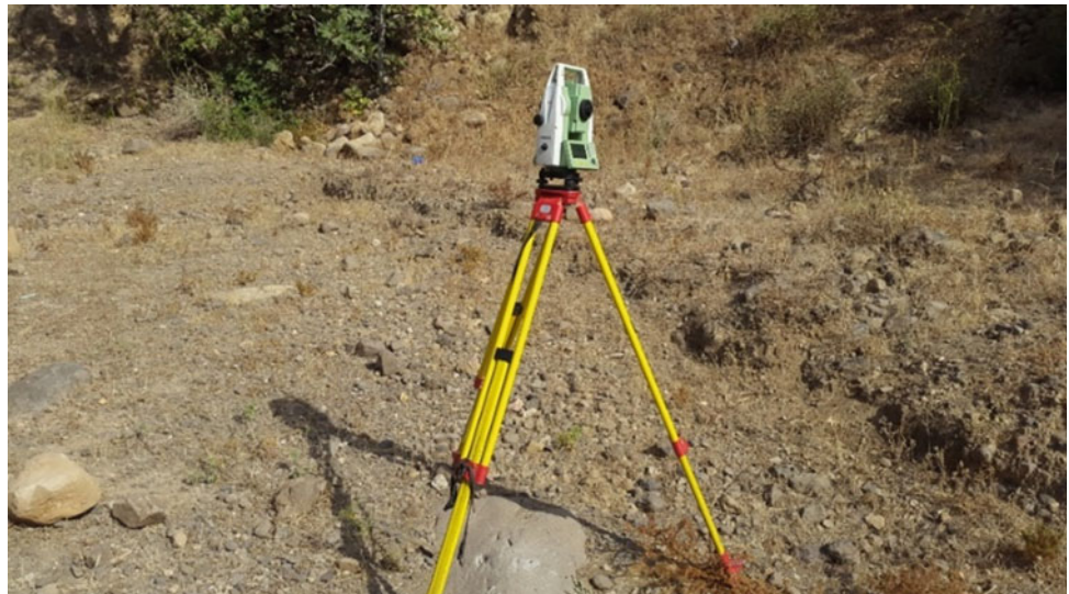
Fig. 2 Total station device used in our study-Leica TS02
