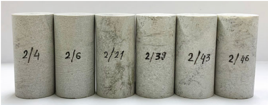
Fig. 22.1 The photograph depicting six limestone samples prepared for the study
