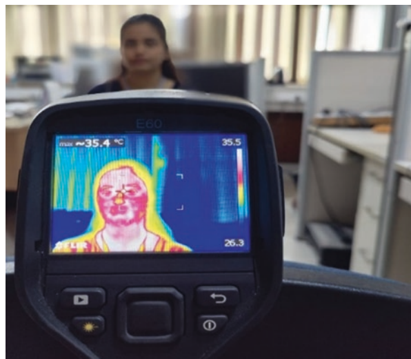
Fig. 2 Shows how to set up thermal imaging properly to analyze persons individually
