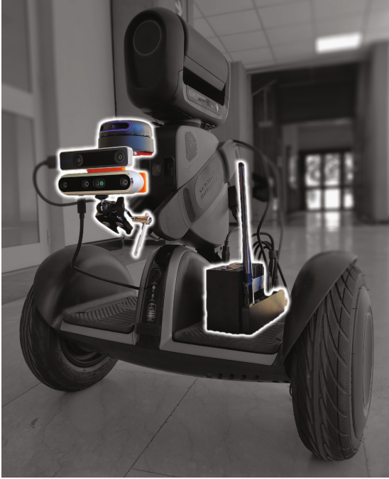
Fig. 1. The proposed MOVING platform, installed on a Lomo robot. The platform consists of a perception module (on the left) formed by an RGB-D camera (bottom-left), a tracking camera (center-left), a 2D Lidar (top-left), and a compact, low-power computational unit (on the right), equipped with a 6-core CPU, a Graphical Processing Unit (GPU) and WiFi connectivity. The sensors are supported by an ad hoc designed 3D printed mount and can be clamped to any robot. The computational unit runs the mapping and navigation software and supports running Deep Learning models on-device.
