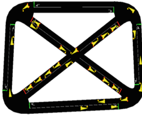
Fig. 6. Sumo-gui view of road with moving vehicles
