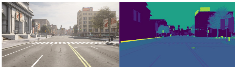
Fig. 2. An example of an RGB camera image (left) and a ground-truth semantic segmentation mask (left) from the training dataset.
