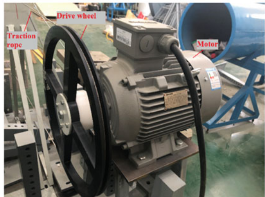
(c) Drive wheel and motor
