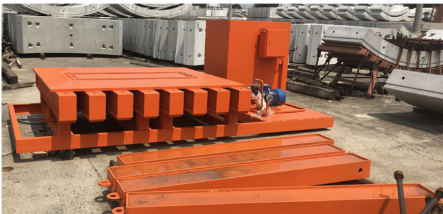
Fig. 4.13 Customized impermeability test device
