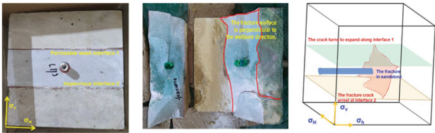
Fig. 35.18 Fracture geometry of #6 after fracturing
