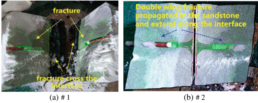
Fig. 35.16 Fracture geometry of the specimens #1–#2
