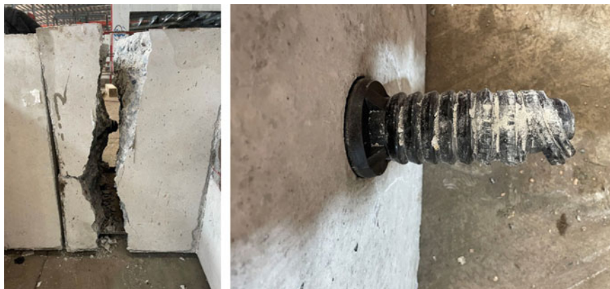
Fig. 5.10 Failure mode of tensile tests
