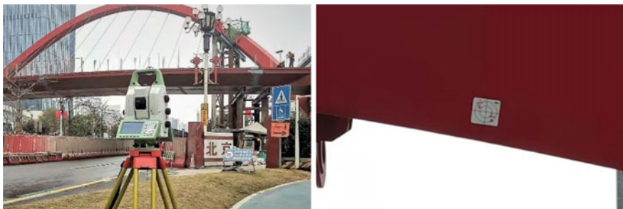
Fig. 76.7 Leica TS60 total station and cross reflector
