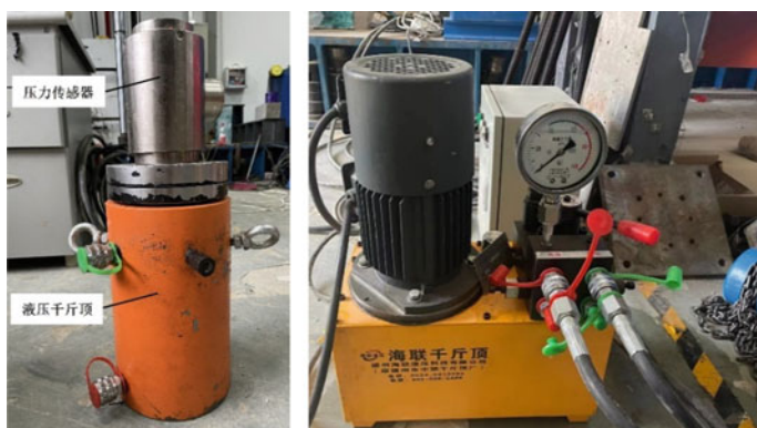
Fig. 5.4 Jack and oil pump of tensile tests
