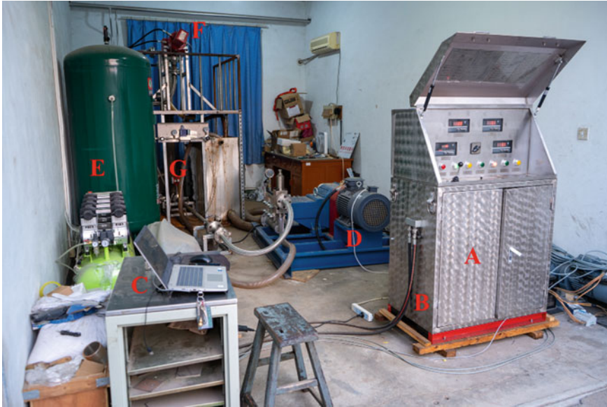
Fig. 47.4 Physical diagram of indoor simulation experimental device: a hydraulic control box; b hydraulic lines; c PID control software; d piston pump; e gas phase injection system (including gas pump and storage tank); f choke; g simulated wellbore
