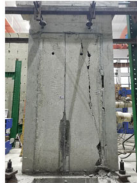
(f) Final condition of Specimen 12
