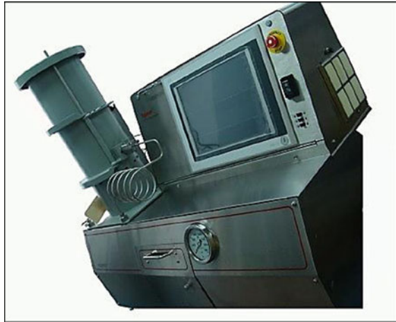
Fig. 29.1 FannIX77 High temperature and high pressure automatic rheometer
