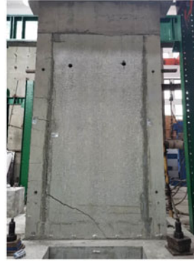
(b) Final condition of Specimen 07
