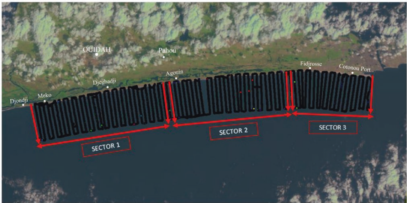
Fig. 2 Graphical representation of the three subsectors of bathymetric measurements on the Djondji-Fidjrosse segment
