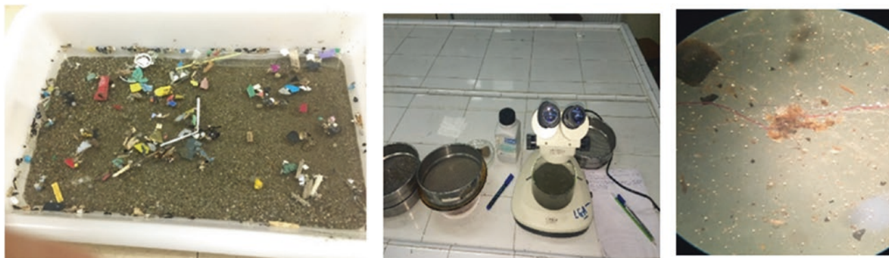
Fig. 3 Images showing the lab work to separate MPs from sediment and quantify them using a binocular magnifier
