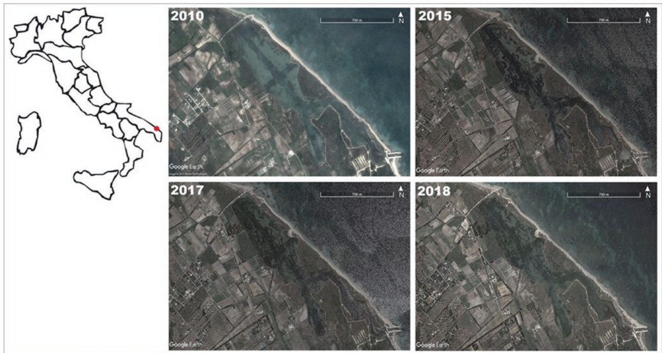
Fig. 1 Multi-temporal evolution of sinkholes in the Acquatina basin (google earth)
