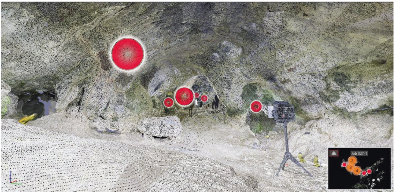
Fig. 1 Lasergrammetry of the Kef EL Baroud cave and its volumetry
