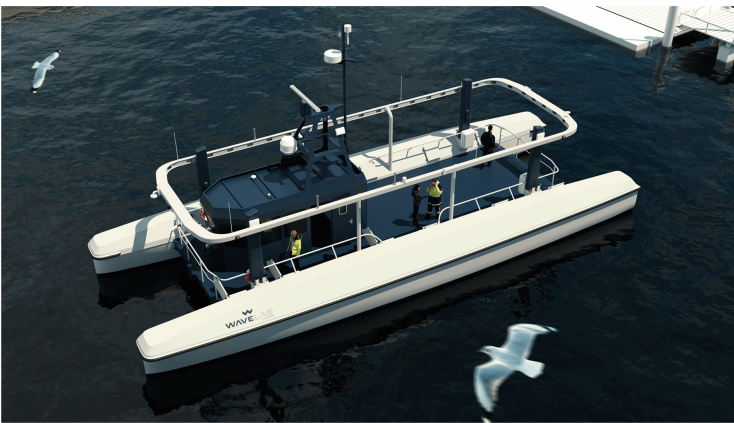
Fig. 1. Design of a 5G remote-controlled passenger ferry “Wavelab” for the Bay of Kiel.
