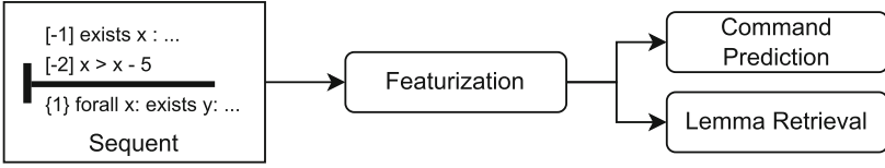
Fig. 1. The CoProver system employs a common sequent featurization, which is used to recommend commands and retrieve relevant lemmas.
