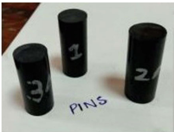
Fig. 18 AC particulate filled epoxy composite samples for abrasive wear test. Reprinted from Prakash et al. [51], with permission from Elsevier. Copyright (2021)
