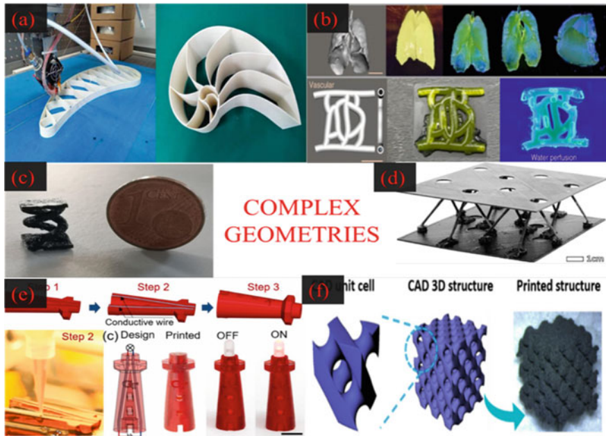
Fig. 4 AM fabricated complex geometries in different science fields a One process cycle printed continuous fiber composite. Reprinted from Hou et al. [101]. Copyright (2018), with permission from Elsevier. b Lung and vascular system printed by digital light processing (DLP) adapted from Kim et al. [90] under the terms of the Creative Commons CC license https://creativecommons.org/licenses/ . c Double helical printed sample adapted from Scordo et al. [102] under the terms of the Creative Commons CC By 4.0. license https://creativecommons.org/licenses/by/4.0/ . d Continuous lattice fiber ultra-light weight composites. Reprinted from Eichenhofer et al. [103]. Copyright (2017), with permission from Elsevier. e Light tower printed by direct ink writing DIW-DLP hybrid system, from printing to a functional device. Reprinted from Peng et al. [104]. Copyright (2021), with permission from Elsevier. f Diamond structure with 60% of porosity (from left to right) unit cell, ordered location Computer-Aided Design (CAD) model, printed high porous structure. Adapted from Rollo et al. [83] under the terms of the Creative Commons CC By 4.0. license https://creativecommons.org/licenses/by/4.0/
