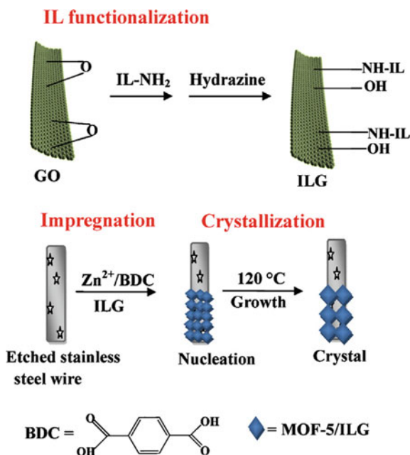
Fig. 8 Schematic demonstration of the in-situ solvothermal growth of MOF-5/ILG on etched stainless steel wire. Reprinted with permission from Wu et al. [136]. Copyright (2016), Elsevier
