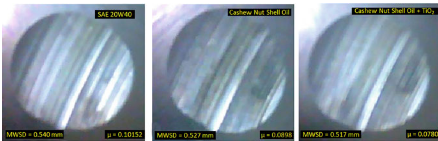
Fig. 5 Tribological performance of SAE20W40, veg. oil, and Veg. oil + TiO 2 using four-ball wear tester
