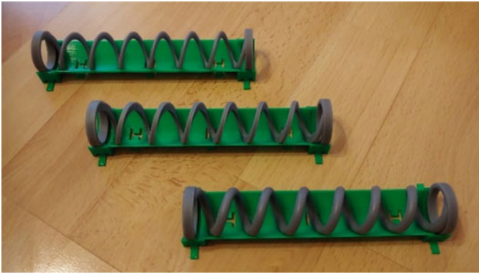
Fig. 5 Elements, after removal of support structures, fixed in forms and prepared for curing with UV light
