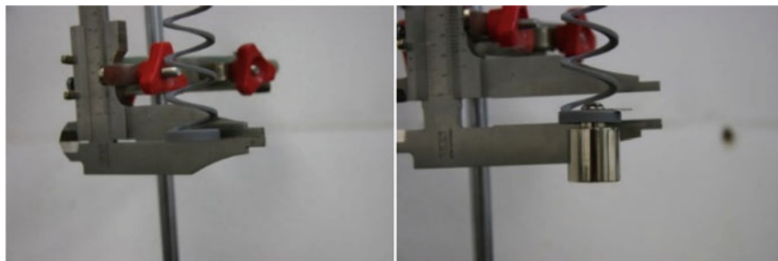
Fig. 7 Fixing and adjusting the spring to the correct height and stretching the spring with a 100 g weight
