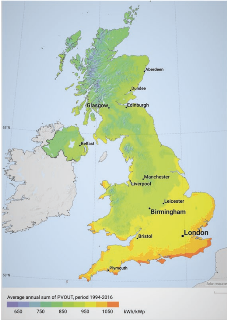
Fig. 7 PV output in kWh per radiation intensity kW_p at various locations in the UK [10]
