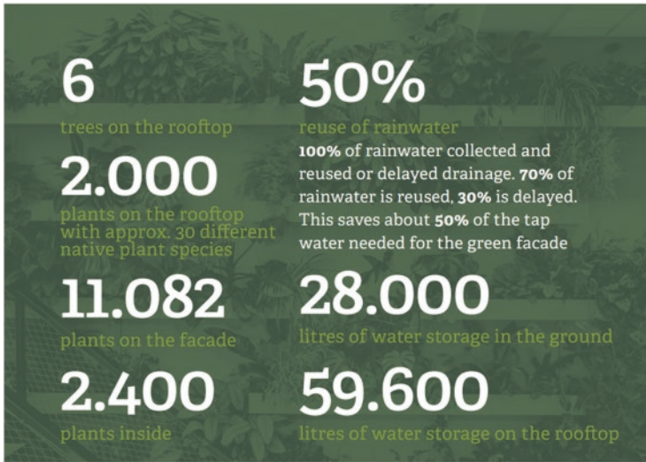
Fig. 20 Integrated design greenery and water storage system
