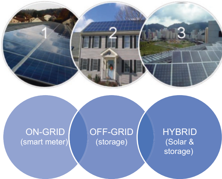
Fig. 50 Different types of PV systems. (Source: Authors, images' credit: (1) Klaus Holl, https://commons.wikimedia.org/wiki/File:Photovoltaikanlage.jpg ; (2) Gary Watson, https://upload.wikimedia.org/wikipedia/commons/8/85/Solar_panels_on_house_roof_winter_view.jpg ; (3) Wing, https://upload.wikimedia.org/wikipedia/commons/2/26/Electrical_and_Mechanical_Services_Department_Headquarters_Photovoltaics.jpg )
