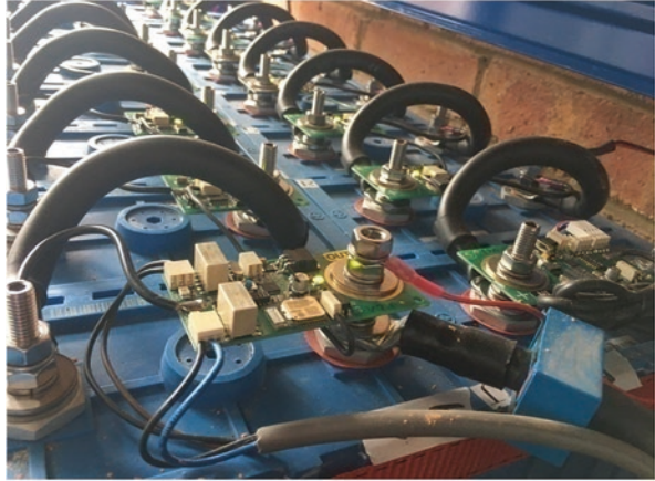
Fig. 16 The CALB 16 × 2000 mAh battery set
