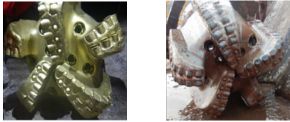
Fig. 6.1 Application effect of PDC bit in hard limestone formation
