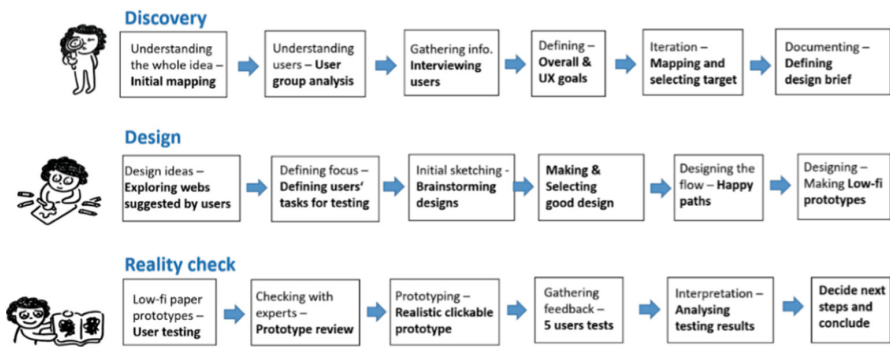
Fig. 1. An overview of the 3 phases and the 18 steps in the UCD Sprint (images © Might Could Studios)
