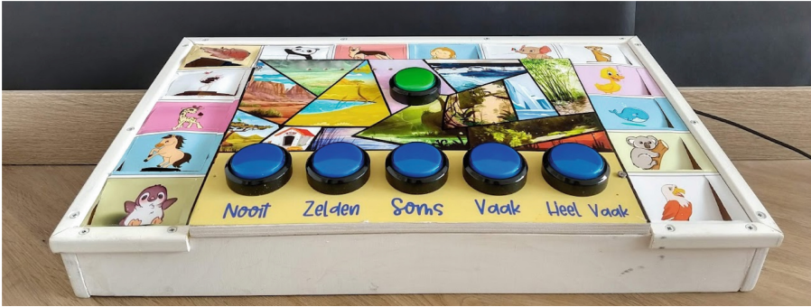
Fig. 1. The Sleep o' Meter: an advent calendar-like perimeter with Lego pieces to be collected and big buttons in the centre for answering questions
