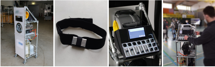
Fig. 1. From left to right: a) The multi-sensory platform prototype with front facing heat, wind and moisture modules; b) the Pavlok shock-band for inducing light pain, c) the interface enabling dynamic change of intensity of each multi-sensory stimuli and d) the MSP in use at a field trial.
