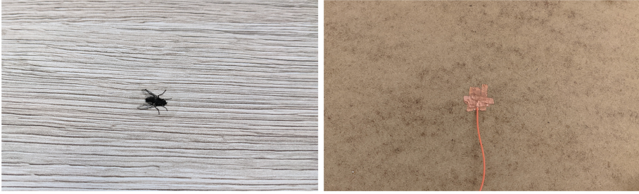
Fig. 1. Left: Wooden board with the graphical representation of a fly. Right: Rear of the wooden board with copper tape at the same position as the fly and copper wire connected to an Arduino, detecting resistance change when the fly is touched.
