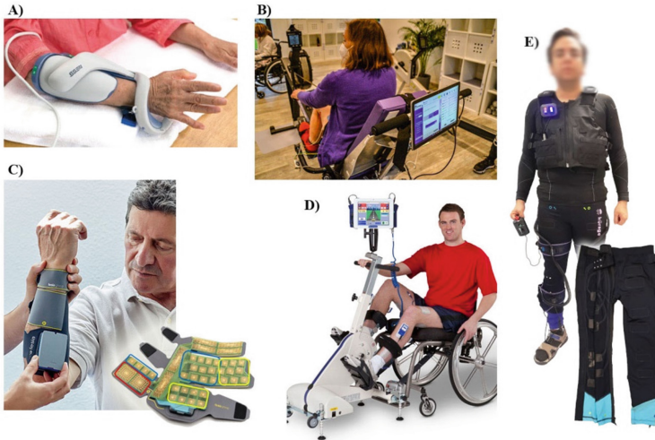
Fig. 4. FES devices: A) NESS H200, Bioness, USA B) Concept 2 rower with Motimove stimulator by Kurage, France, C) Feasia Grasp, Fesia Technology, Spain, D) RT300, Restorative Therapies, USA, E) Neuroskin, Kurage, France.
