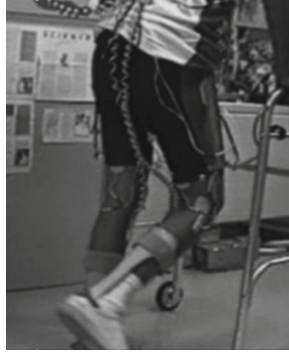
Fig. 2. Paraplegic patient walking with automatic FES gait based on closed-loop control with joints angle and GRF sensors
