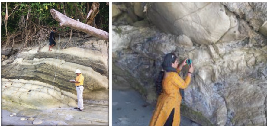
Fig. 23.2 Measuring the dip of the bedding plane on the rock outcrop of the shore cliff at Havelock Island (Archipelago formation)
