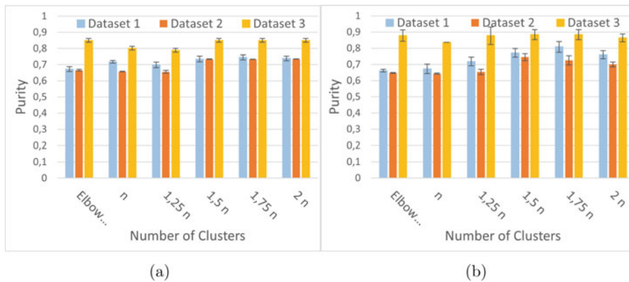
Fig.10 K-means clustering (a) and GMM clustering (b) purity for different specified numbers of clusters for different data sets
