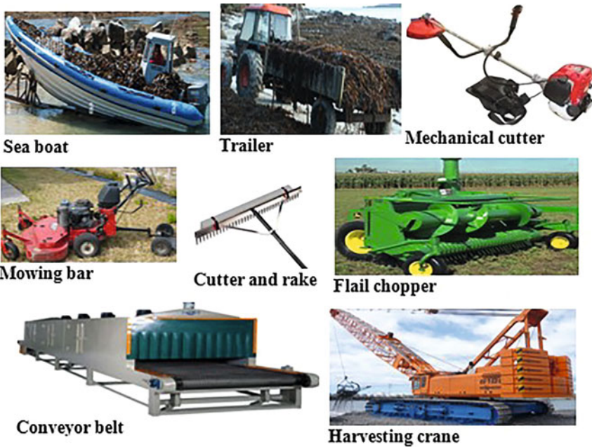
Fig. 3 Mechanical equipment for seaweed harvesting
