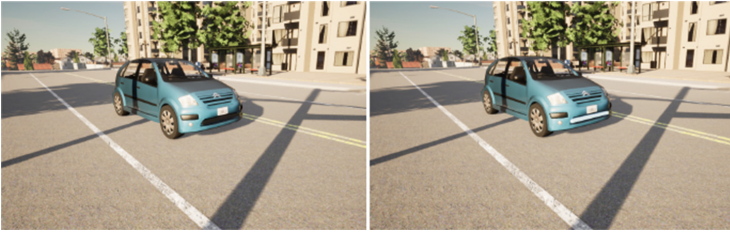
Fig. 3. Left: vehicle with eHMI deactivated. Right: vehicle with eHMI activated [8].
