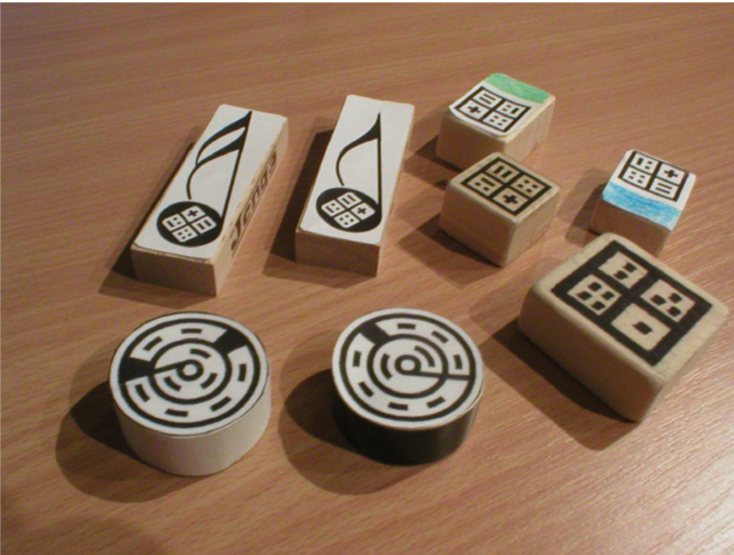
Fig. 5. The fiducial markers of D-Touch . The picture is taken from [20].
