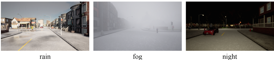
Fig. 5. Overview of the used weather conditions. The grayish sky, falling water drops as well as water puddles on the road are characteristic for rain . In the case of fog , fine water droplets cover the image, and it is especially tough to see in depth. Night images are characterized by many dark areas, with streetlights and vehicle lights illuminating the scenes.
