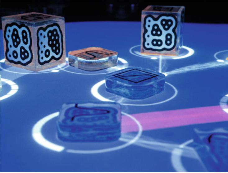
Fig. 4. The fiducial markers of the Reactable . The picture is taken from [23].
