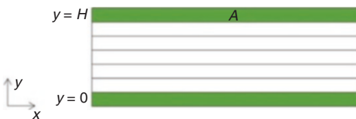
Fig. 4 Two-plate model: fluid layers between two plates at rest
