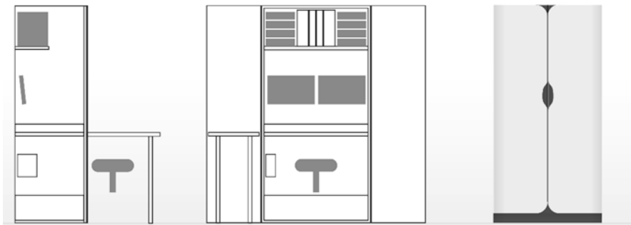
Fig. 28.16 Hybrid office terminal (model 3), which features a height adjustable and tiltable desktop, a foldable desk serving as a large working area with additional space, a footrest, and an integrated seat
