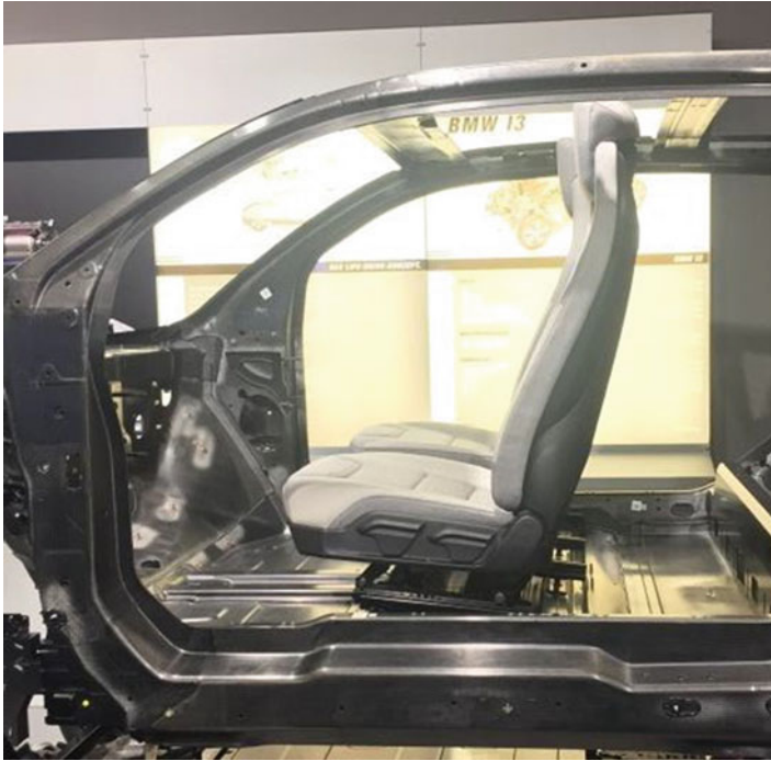
Fig. 28.6 Thin seat shells for an e-car
