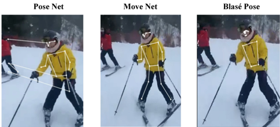
Fig. 4. The difference between the three models when there is more than one person on the frame.
