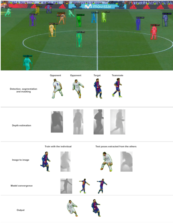
Fig. 3. The proposed framework step by step. From top-to-bottom, we start with player detection, segmentation, and masking. Next, we obtain a sprite dataset and keep our target player separately - in this case, Lionel Messi. Then, we proceed with depth estimation for all our extracted sprites. Lastly, we train an image-to-image generative model with our individual-target data and test it with the collective depths from poses across the pitch. Our result will be the sprites of Lionel Messi in novel target poses.
