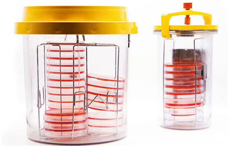
Fig. 4 Commercially available anaerobic jars used for the cultivation of anaerobic microorganisms
