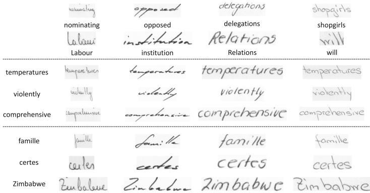
Fig. 3. Synthetic handwritten images conditioned by different writer IDs with different words. Top: real samples with corresponding words from IAM writers 001, 002, 023 and 027, respectively. Middle: synthetic samples of words that are seen in IAM training set. Bottom: synthetic samples of out-of-vocabulary words.
