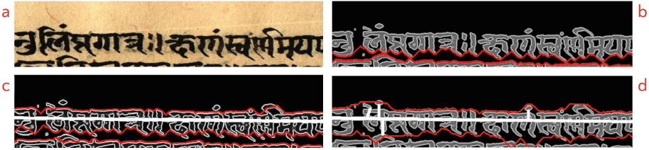
Fig. 6. (a) A fragment from the top portion of a manuscript (b) Seams generated with Gradient and Smoothing Map, but without using scribble – the upper line boundary is missing (c) Seams when scribble is also added – upper line boundary is obtained, but diacritics are missed (d) Seams when Diacritic Map is also included – line boundaries properly enclose text and associated diacritic components.
