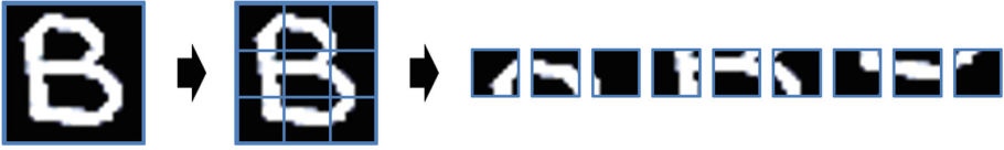
Fig. 2. An example of how ViT turns an image of a character into a sequence of patches.
