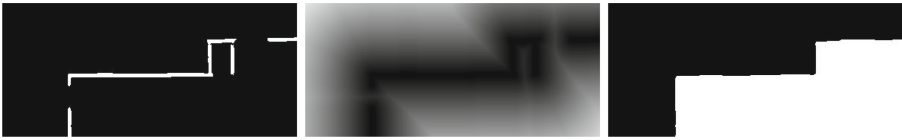
Fig. 5. From the left: detail of unclosed contour prediction, its euclidean distance transform, the result after watershed
