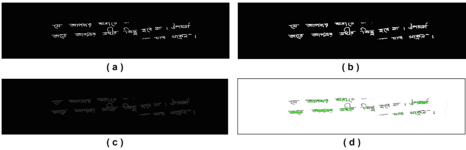
Fig. 7. Preprocessing and Hough line detection of sample resized line image represented in Fig. 6; where a) Binarization, b) Morphological Dilation, c) Canny edge detection, and d) Detected Hough lines using PHT.
