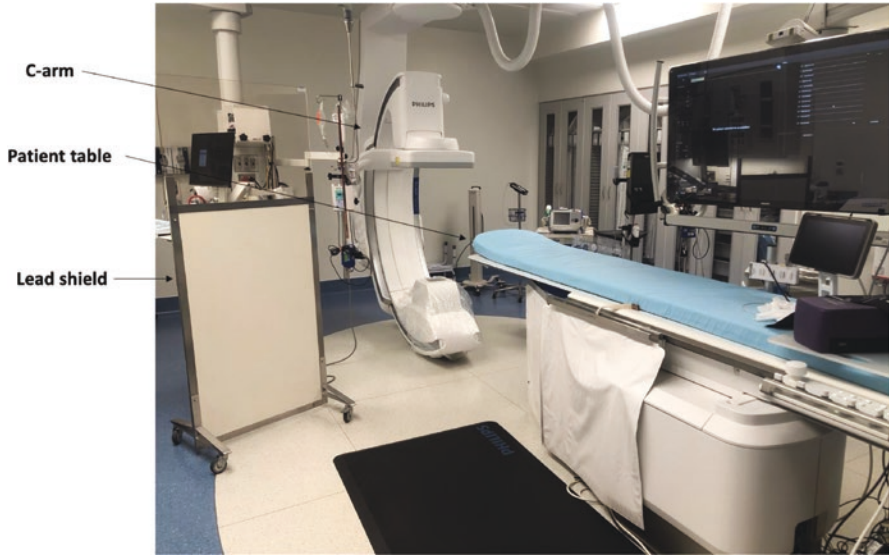
Fig. 6.1 Standard setup for the cardiac catheterization laboratory
