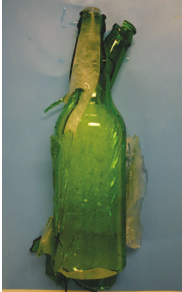
Fig. 1 A bottle filled with water left to freeze will shatter the glass by expanding ice crystals
