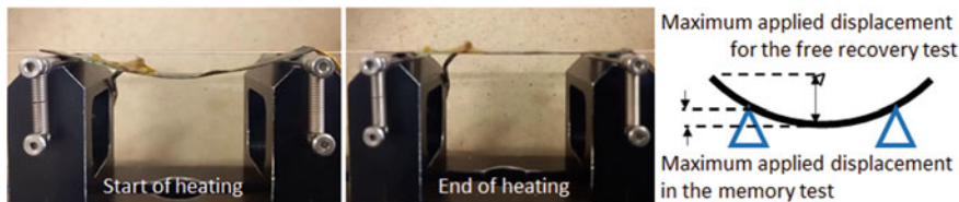
Fig. 9 Initial and final configuration of the SMPC laminate device during the free recovery test (case of 10 mm of inflection by bending) and difference between the considered maximum displacement in the memory and free recovery test
