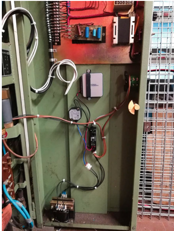
Fig. 3 Modification of the resistance spot welder for remote controlling
