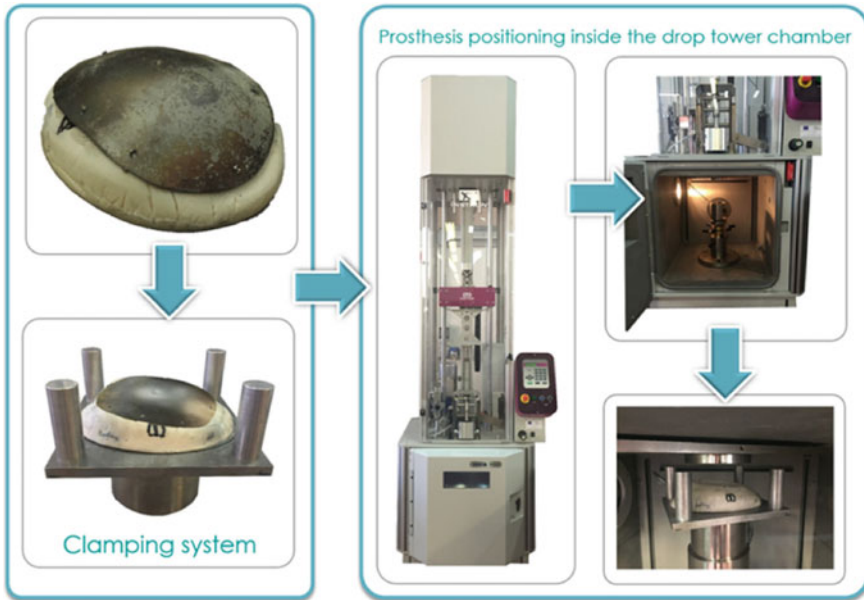
Fig. 17 Definition of a pre-clinical protocol based on impact loading using a drop test tower
