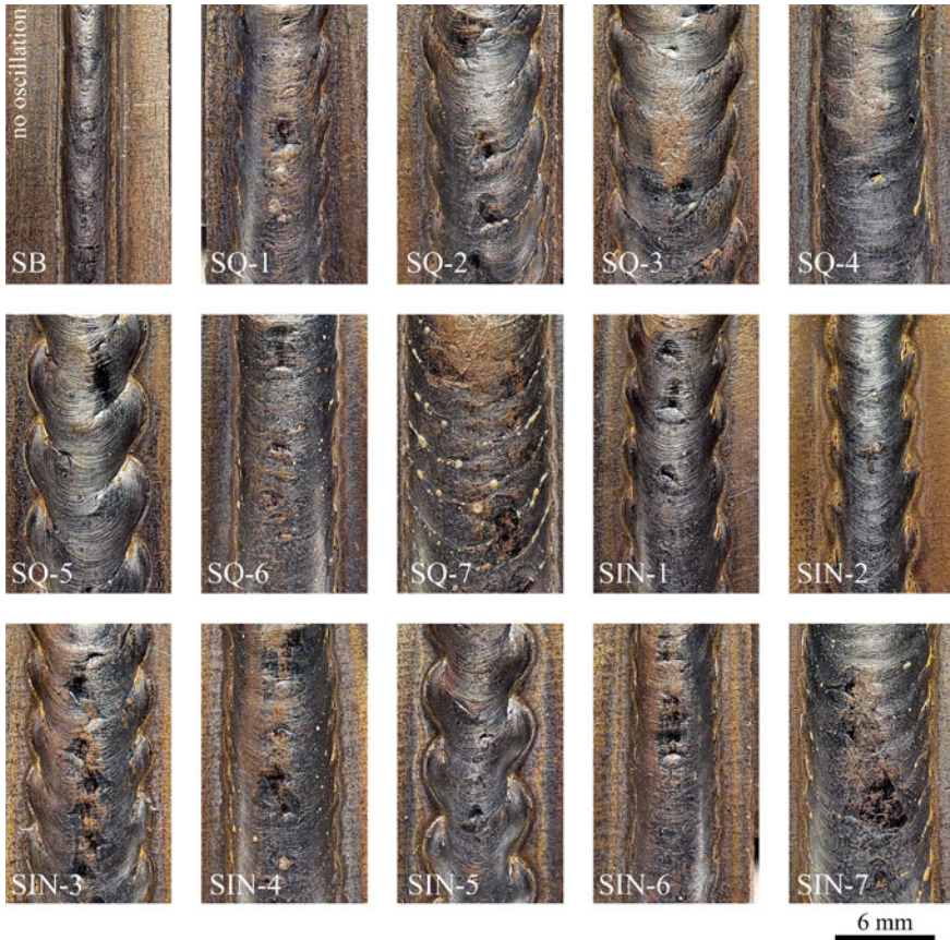
Fig. 2 Aspect of the narrow bead without oscillation (SB) and the oscillated beads
