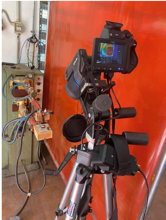
Fig. 7 Picture of the IR camera positioned over the equipment for temperature measurement
