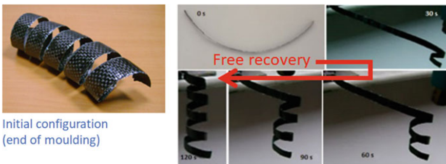
Fig. 2 Free recovery of a CFR-SMPC spiral (results from the Horizon 2020 SMARTFAN project, GA No.760779)
