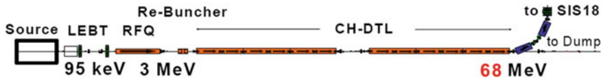
Fig. 3.28 Schematic layout of the FAIR p-Linac [20] (the original output energy 70 MeV was changed to 68 MeV in 2017)
