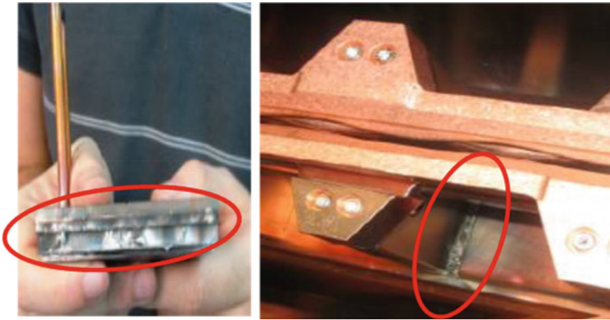
Fig. 1.14 One burnt connection between a tuning plate and a stem of the SARAF RFQ [51]
