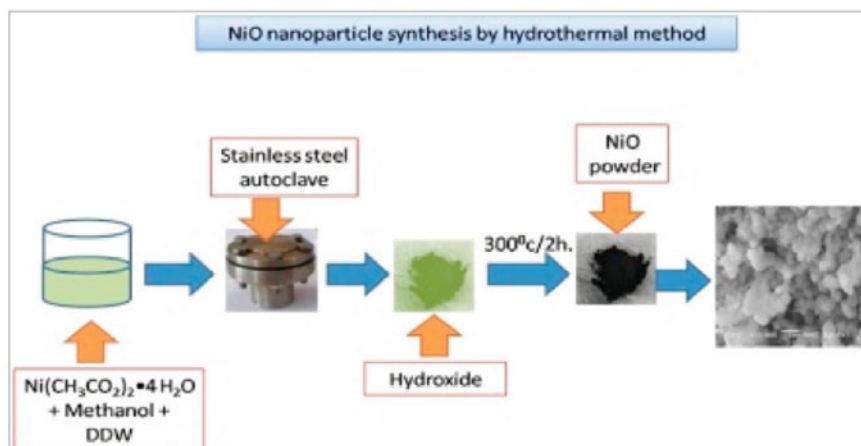
Fig. 12.9 Hydrothermal techniques for the preparation of NiO nanoparticles. Reprinted the figure with Copyright (2020) permission from Elsevier et al. [33]
