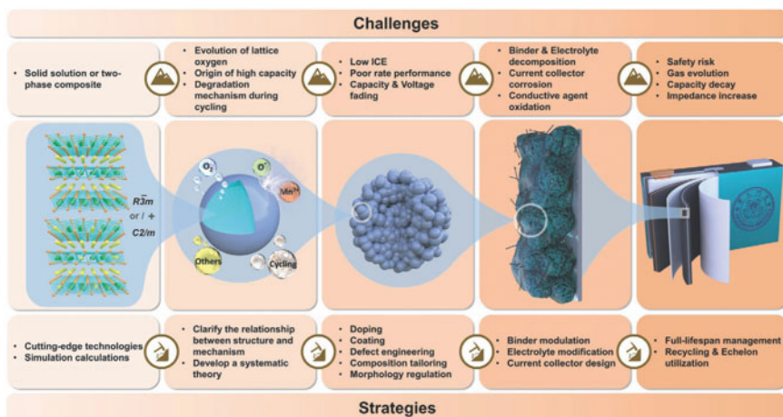
Fig. 14.11 Schematic diagram summarizing the challenges and strategies of LRM cathode materials in different stages from crystal structure to practical application. Adapted with the permission ref. [121] © 2021 Wiley-VCH GmbH
