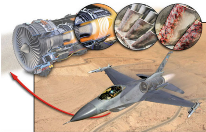
Fig. 3 Military aircraft flying during a sand storm in an arid region. Image insert-mineral dust particles passing through the gas turbine and corroding the ceramic coatings and metallic surfaces of the hot section components [8]
