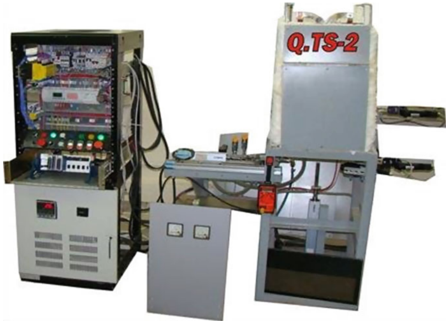
Fig. 6 The quick thermal shock installation within the National Institute for Aerospace Research “Elie Carafoli”—INCAS Bucharest [34]
