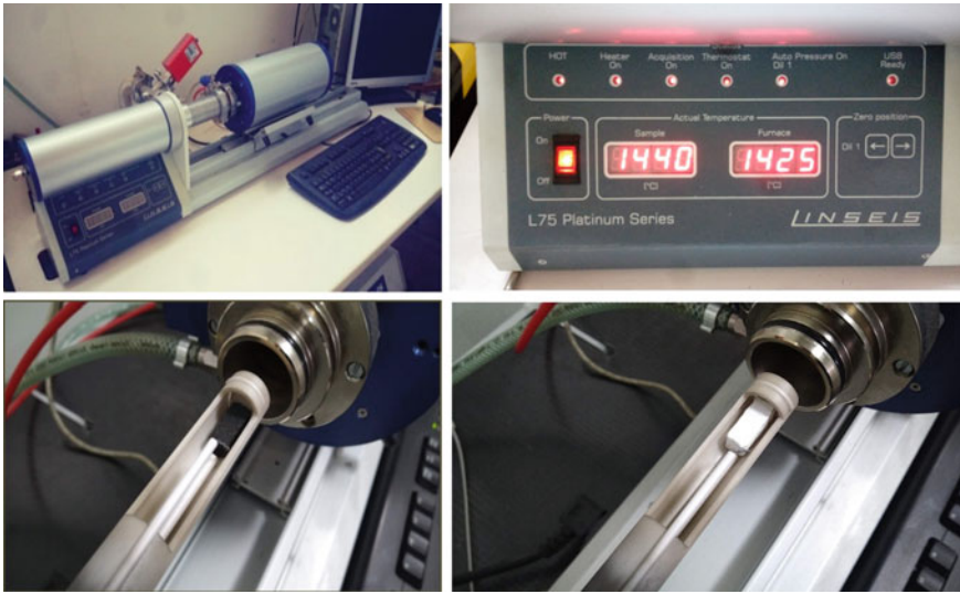
Fig. 4 CTE measurement setup: dilatometer L75HX1600 in closed configuration, device display showing sample and furnace temperatures, pushrod/sample (left—SiC; right—ALP) arrangement before the test. [26]
