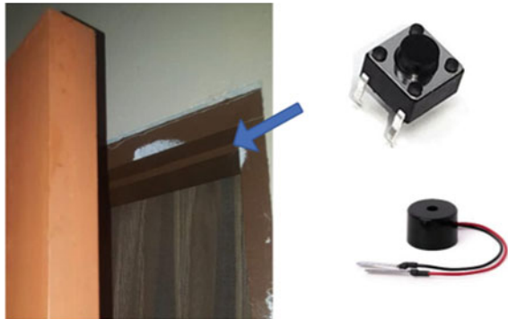
Fig. 5 Example on placing/ locating push button to door
