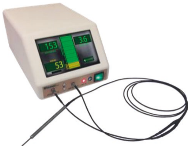
Fig. 6.1 PTeye™ (Medtronic, Minneapolis, MN, USA) near-infrared auto-fluorescence probe system. (Image from PTeye™ brochure https://www.medtronic.com/content/dam/medtronic-com/products/ear-nose-throat/pteye/documents/pteye-product-brochure.pdf )
