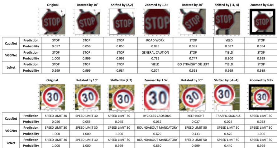
Fig. 4 Predicted classes and their probability associated with the prediction confidence, comparing the CapsNet, VGGNet, and LeNet, under different affine transformations applied to two examples of the GTSRB dataset [51]
