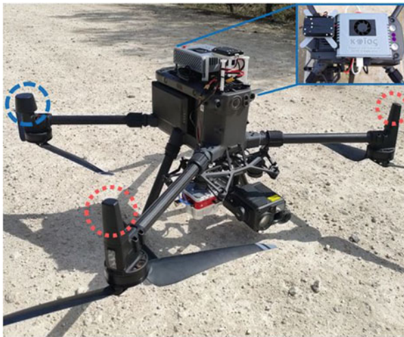
Fig. 3 UAV equipment with the embedded system for testing the proposed MELETI system architecture. It consists of a DJI Matrice 300 RTK UAV, the RGB and thermal DJI Zenmuse H2OT camera (right downward gimbal), the multispectral MicaSense Altum camera (left downward gimbal), and the NVIDIA Jetson Xavier NX embedded system (top of the UAV; figure inset). Blue dashed and red dotted circles indicate the differential RTK and the transmission antennas, respectively
