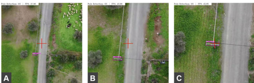
Fig. 10 Power infrastructure pole detection and position correction. (a) Real-time pole detection using the tiny YOLOv4 on the NVIDIA Jetson Xavier NX embedded platform. (b) Pole position correction by aligning the image center (red cross) to the center of bounding box (pink). (c) Spatial coordinates recorded using multiple GNSSs as the accurate coordinates of the current pole
