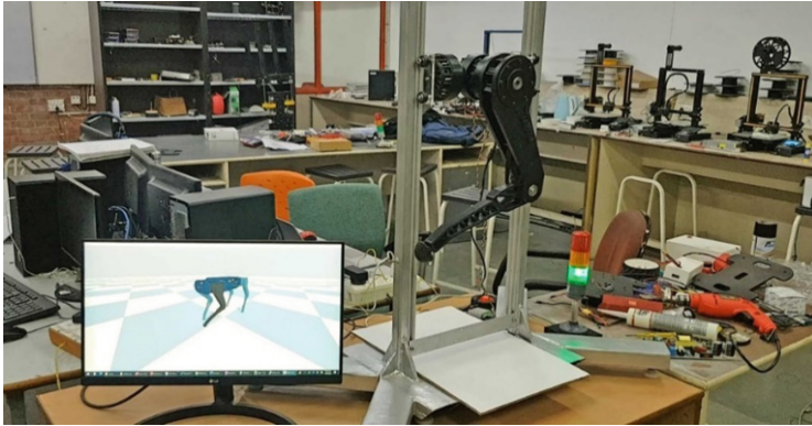
Fig. 9. The real robot leg mounted on the test rig and the simulation environment using PyBullet
