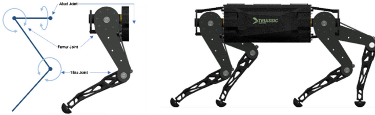
Fig. 6. Leg configuration of “Stego” the real quadrupedal robot built for our experiments
