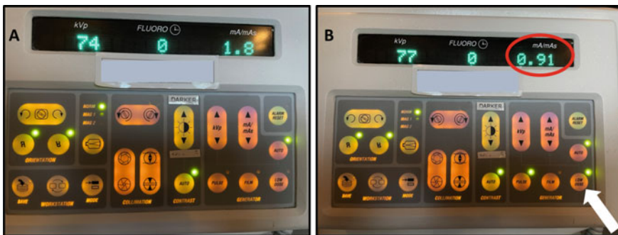
Fig. 3 (A) C-arm settings in standard automatic exposure control. (B) Depression of the low dose button (white arrow) results in reduction of dose output by half as reflected by the mA (red circle)
