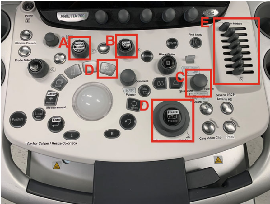
Fig. 3 Typical ultrasound machine setting controls including A) Gray scale mode, B) color doppler mode, C) frequency and depth, D) gain, E) time-gain compensation and F) field of view
