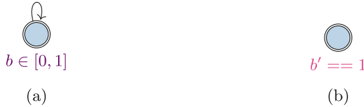
Fig. 5. (a) A Specification, modelling the battery capacity of the light controller, whose timing behaviour is defined by the specification depicted in Fig. 2. It consists of a single mode, the initial mode, and is defined over the global resource b . It invariantly requires that the battery capacity never exceeds 1 unit of energy and is never saturated beyond depletion. Note that any and all discrete transitions are allowed, captured by the self loop. (b) A Specification, modelling a power supply. It consists of a single mode, the initial mode, and is defined over the global resource b . It does not admit any discrete behaviour, however it defines a constant charging of 1 unit of power per time unit.
