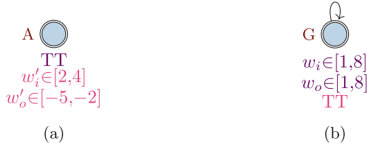
Fig. 9. (a) An RHA modelling our assumption on the environment. We assume that the input reservoir gets filled by a rate in the interval [2, 4] and that the output reservoir gets saturated by rate in the interval [-5, -2] . Additionally, we assume that the environment never saturates the usage reservoir, thereby completely delegating that responsibility to the system from a modelling perspective. (b) Another RHA modelling our guarantee on the system if the assumption is fulfilled. We guarantee that the capacity of both the input and output reservoir stays in the interval [1, 8] . Additionally, we guarantee that at any time, a discrete event can occur, as long as it performs no resets.
