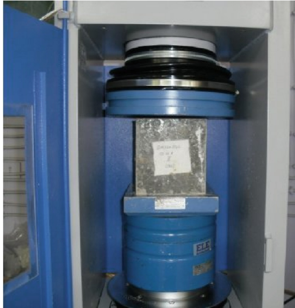
Fig. 2. Representation of concrete compressive strength test [8].
