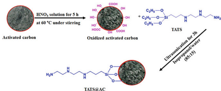
Fig. 6.2 Synthesis of TATS@AC [Reprint with Permission; Naushad et al. 2020]
