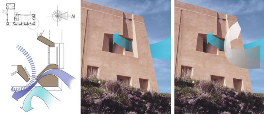
Fig. 3 Wind deflectors at the northeast edge of the upper storey
