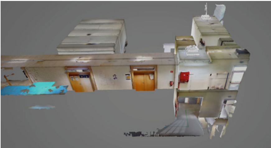
Fig. 9 Matterport 3D.obj export, scanned with the leica BLK360 laser scanner, shown in windows 3D model viewer
