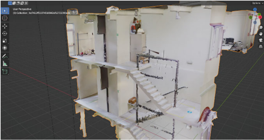
Fig. 10 The same model as Fig. 8 but imported into blender, to gain a better view of the retrieved data from matterport
