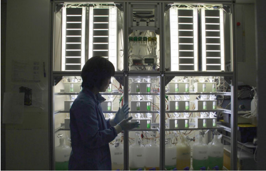
Fig. 1 Detail of the fully inoculated Living Architecture ‘wall’ and apparatus installed at the University of the West of England, Bristol, the Living Architecture project, 2019. Photography by Rolf Hughes © Rolf Hughes. An array of fifteen bioreactors within the ‘living’ wall that houses microbes in a large apparatus about the size of a bookcase
