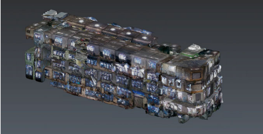
Fig. 8 Complete watertight mesh of the reduced product development campus building using leica cyclone REGISTER 360 and cyclone 3DR
