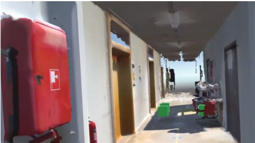
Fig. 2 VR application in unity with the imported mesh of the campus' 3rd floor as an interactable environment
