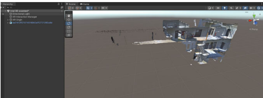
Fig. 11 3D model export result, imported into unity. To use as a virtual environment in multiple user contexts
