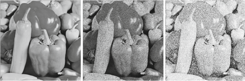
Fig. 1. Left: Original image; Center: Corrupted image containing 50% impulse noise; Right: Locations of detected noisy pixels in white.
